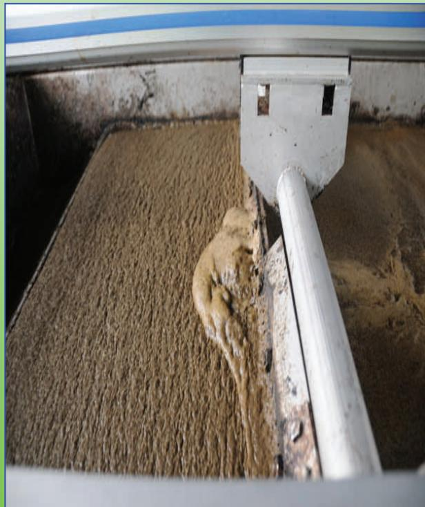
The combination of Ozone treatment process as a POME polishing plant, has been tested in operation for more than 9 months using the pilot R&D polishing plant, and results have shown to be able to treat the POME from the algae or aerobic pond discharge water to achieve the 20ppm  $BOD_3$  limit.
